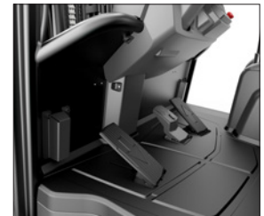
Dual pedal system - forward and reverse.
